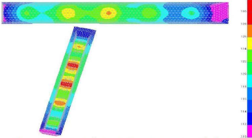
Image 14: Simulation of heat output on daytime running lamp design without pins
