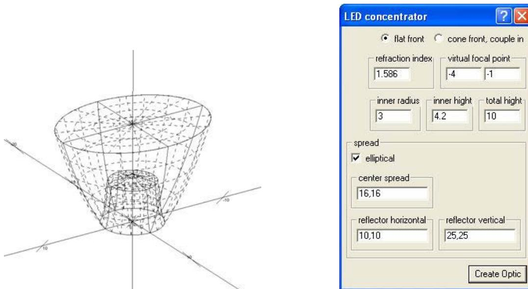
Image 6: Design of the basic lens geometry within Lucidshape with the aid of one of the application tools
