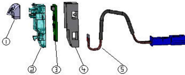
Image 1: Exploded view of a typical ambient lighting assembly consisting of lens (1), cap with integrated light guide (2), electronics pcb with light source (3), housing (4) and cable assembly (5)
