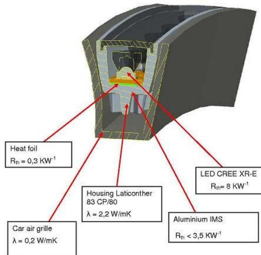
Image 13: Section through a daytime running lamp showing the individual parts required for thermal simulation
