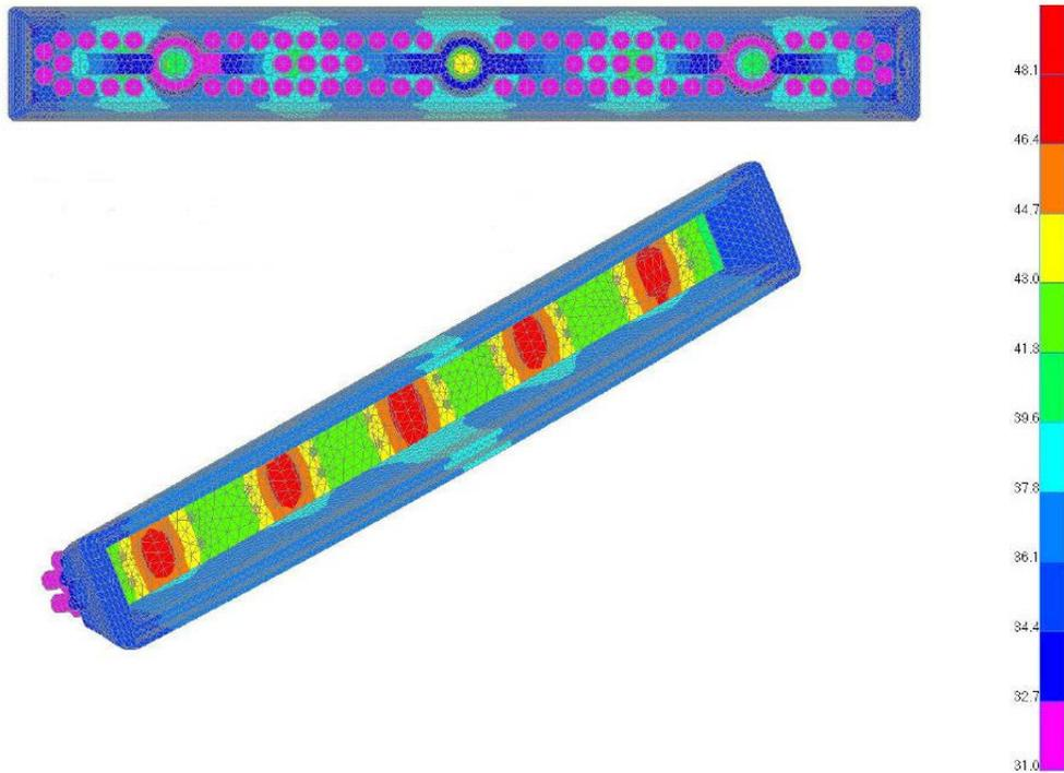
Image 16: Simulation of heat output on daytime running lamp design after the introduction of pins
