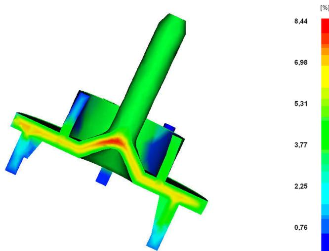
Image 12: Cut through a light guide simulated with mould flow analysis showing volume shrinkage
