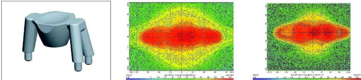
Image 10: Effect of sink mark on light output; LHS Simulation with a light guide without sink mark, RHS with sink mark
