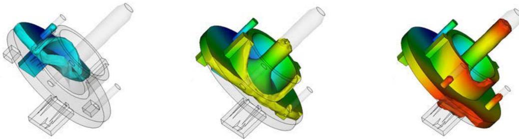
Image 11: Mould Flow Analysis on a light guide showing plastic filling stages with time
