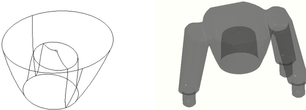
Image 8: Light guide after initial light simulation (LHS) and final production part (RHS)
